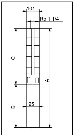
101 mm = Maximum diameter of pump inclusive of cable guard & motor.
